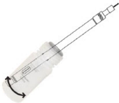
**✓ TIP:** With the correct fill level, and the instrument held at a 45° angle, the air bubble in the Cal Cup will not intrude into the conductivity sensor.
