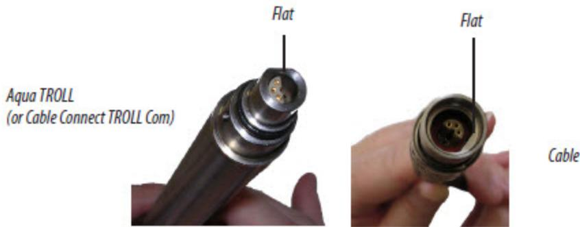
Note the pins on the instrument connector (one on each side) and the slots on the cable connector (one on each side).
