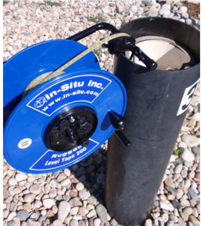
Figure 4. Rugged Level Tape 200 installed in well
