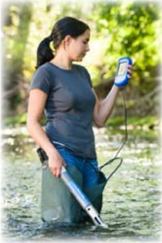
Choose from several field-ready sensors. The selected sensor set will determine the diameter of the TROLL 9500—sub-2 inch or sub-4 inch.
